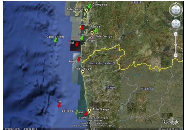
Marine observation grid (green: present grid; red: to be implemented during RAIA) - IIM Fulmar Buoy circled
