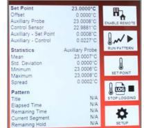
of the 5600 Series Bath Interface is a true Metrology Based Interface providing: fundamental control via a proportional-integral-derivative (PID) digital overlay; and storing and accessing 17025 required Metrology Based data on temperature, stability and bath operation. A true Metrologist tool!
