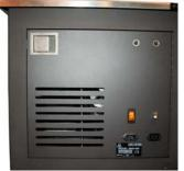
maintenance. The circulation pump, cooling unit and electronic hardware are located in a separate compartment beside the tank with a convenient access panel to provide full and unimpeded access. This compartment is EMI shielded from the bath tank, which in turn has its own EMI shield.
