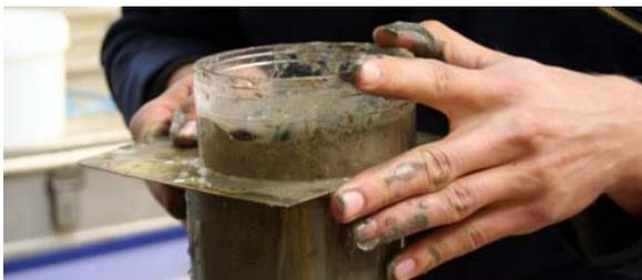
The research team used a megacorer, supplied by OSIL, to collect sediment cores from 500, 700 and 900 m in the Darwin Mounds area, which were then incubated after addition of different quantities of  $^{13}\text{C}$ -labelled fresh organic matter into the samples.
