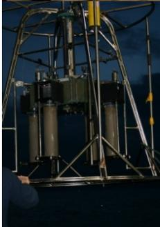
The rugged frame of the corer is made from 316 stainless steel and the core tubing itself can be manufactured from acrylic, poly carbonate or stainless steel, depending on the requirements of the customer. With a deployment rate of approximately 1 metre per second on the descent, coupled with a retrieval rate at winch speed, the corers are ideal for rapid assessment work.
