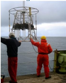
The Mega Multiple Corer used on the cruise is a hydrostatically damped multiple-corer (penetration rate ~1 cm/s), designed to collect high quality undisturbed samples of surface sediments, including the sediment/water interface and overlying supernatant water. Each of the four multiple corers available, Mega, Maxi, Midi and Mini, provide a simple and reliable way of collecting the most accurate sample possible by eliminating the bow wave generated by traditional corers.
