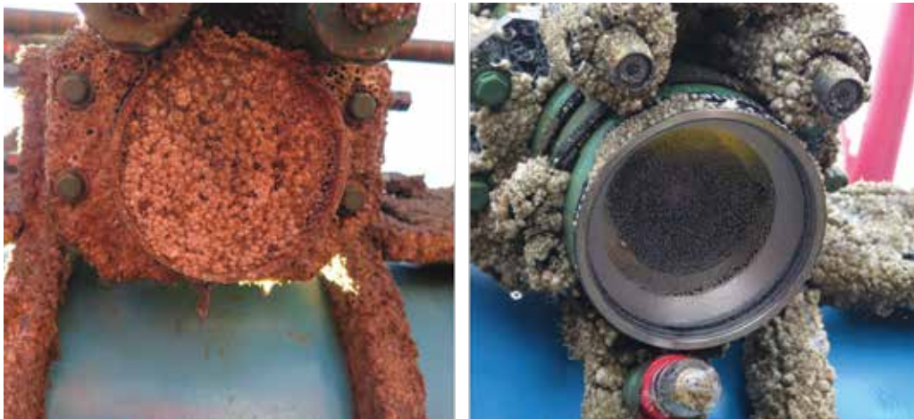
Cameras deployed for six months, without Cabled UV (left), and with Cabled UV (right). Note the incidental protection of the lights above the lens on the camera to the right. (Images courtesy of Oregon State University)
