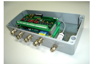
Barometric pressure sensor in OMC-183 housing
